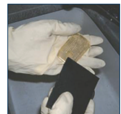
Removing support material
