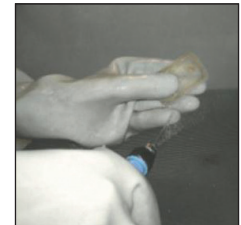
Removing support material
