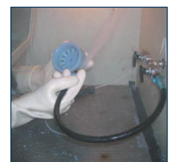
Cleaning a model with the WaterJet
