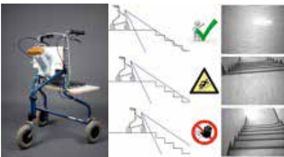
Figure 1: (left) prototype with stereo camera; (right) (top) a safe situation, (middle) a warning situation, the danger is located in the half upper part of the image and (bottom) a dangerous situation.
