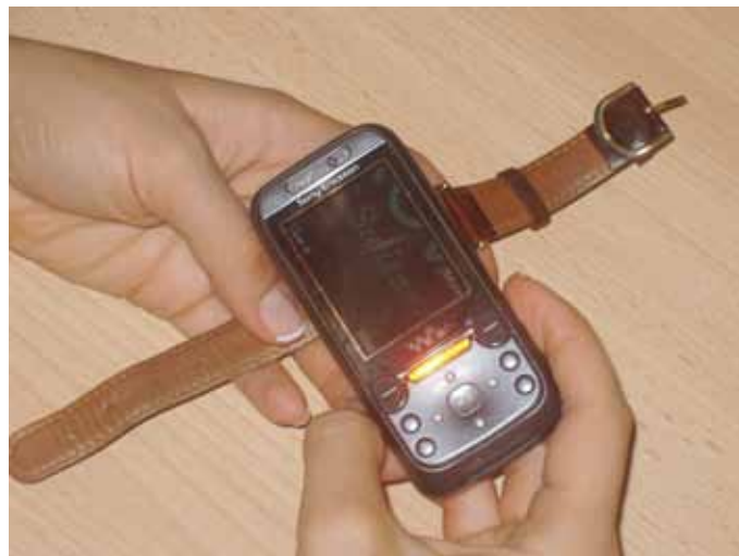
Figure 4: Watch authentication based on the surface microstructure acquired by a mobile phone (SNF Prof Boursier and ECRYPT projects).
