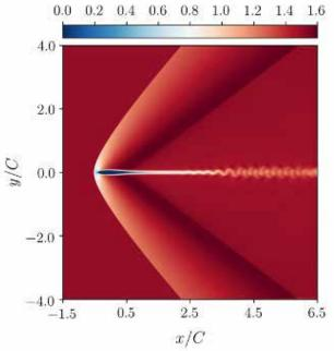
Figure 3: Simulation of supersonic flow around an airfoil, with a shock front
