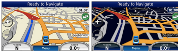
The day and night interfaces in the GARMIN Zumo 660 adapt the interface color so the user isn't blinded with a bright light.
