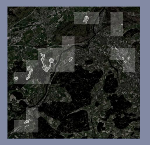
From aerial images to quarries inventory and evolution survey Combining detection polygon with geological data to identify the exploited resources in an automated way
